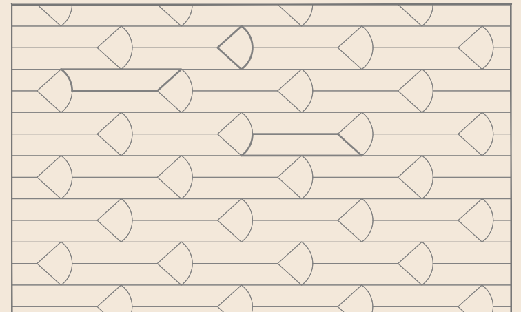
Eco - Posa / Installation 302 Elementa by Marco Piva 140x780mm, 140x780mm, 280x227mm
